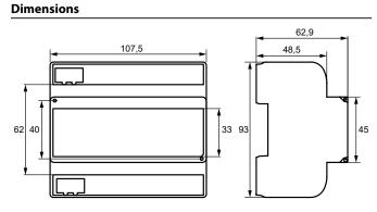
Dimension diagram (in mm)
